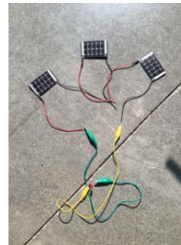
Connecting solar modules in series to light red 12v LED
