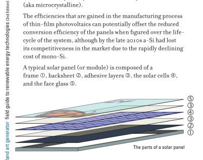
The face glass can be clear or it can be tinted any solid color, be fritted with patterns, or be applied with a high transmittance printed film, like the artwork, La Monarca, on the following spread (film applied over mono-Si).
