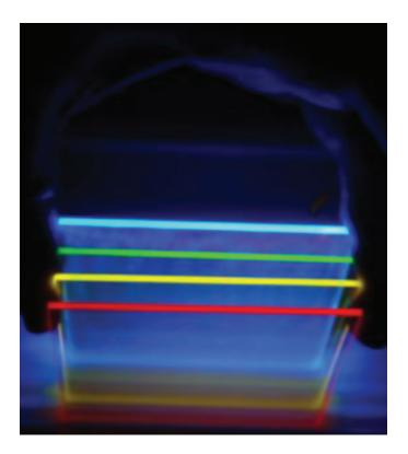
The application of special dyes to the surface of a pane of glass or plastic can cause a certain spectrum of light to be diverted at concentrated levels directly to the edges of the glass, where it can then be collected by a solar cell that is calibrated specifically for that wavelength. All other light wavelengths continue uninterrupted through the glass pane, which appears almost completely transparent.
